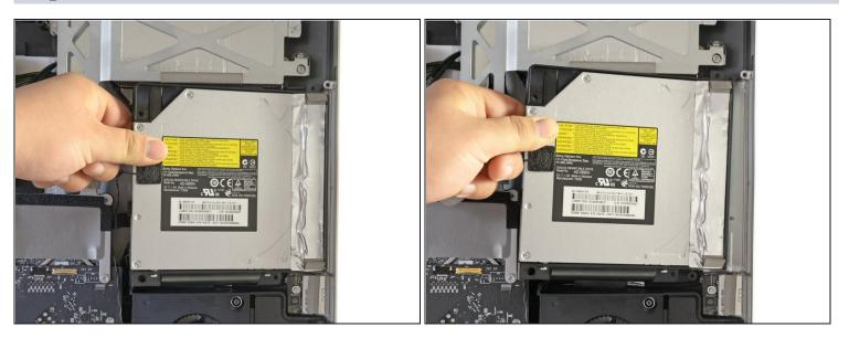
• Slightly lift the left edge of the optical drive and then pull it to the side to release the centering pins.
