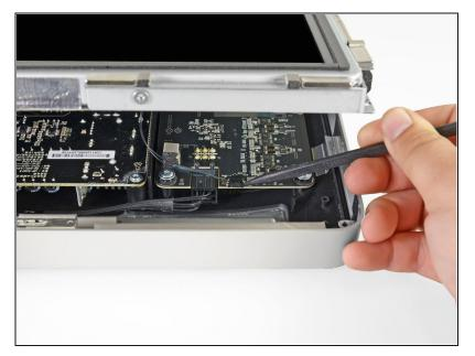
Disconnect the vertical sync cable in the upper left corner of the screen. Use the tip of a spudger to push on the connector's side tabs and gently walk it out of its socket.
