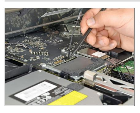
Use the tip of a spudger to disconnect the display power cable next to the display data cable.
