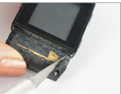
Scrape away the glue beneath the hard shell portion of the band to reveal the GPS.
