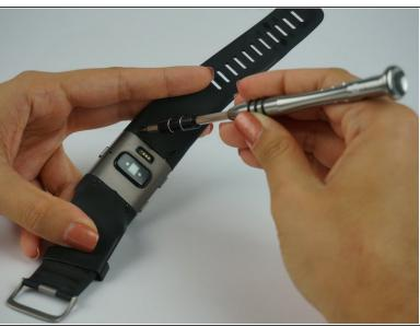
Unscrew all four black 3 mm screws on the underside of the watch using a T5 screwdriver.
