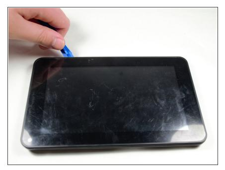
Remove the back of the device using the Plastic Opening tool by placing it between the front and back panel and gently prying them apart.
