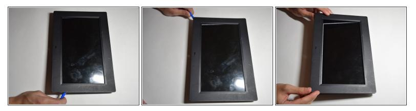
• Using the plastic opening tool pry off the clips all around the frame. You will hear a popping sound for every clip
