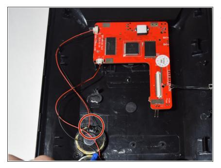
Disconnect the wires off of the old speakers and solder the old wires onto the new speakers.
