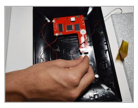
Disconnect the red and black cable connecting the screen to the motherboard by just pulling it out. To reassemble your device, follow these instructions in reverse order.
