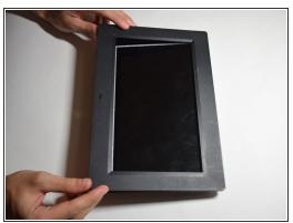
Using the plastic opening tool, pry off the clips all around the frame. You will hear a popping sound for every clip
