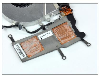
(i) After scraping off the solidified thermal paste, a residue is still present on the copper core(s).
