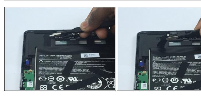
Remove any tape that may be holding down the speakers or wires in place.
