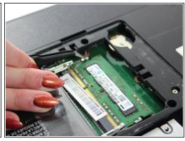
Using the curved tweezers from the Precision Tweezers Set grab and pull the metal clips away from each side of the RAM.
