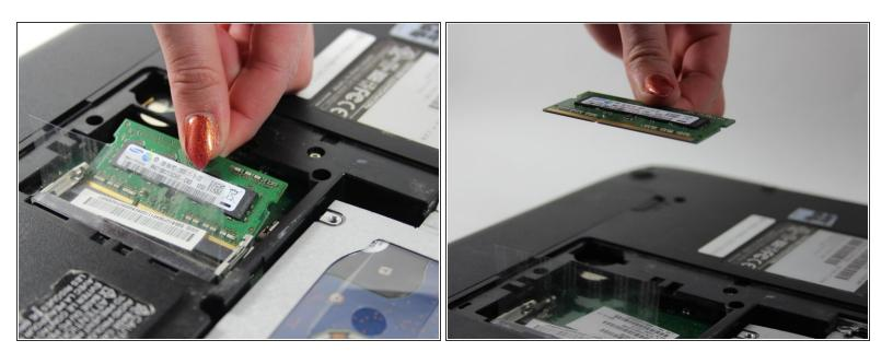
Now the card is free to remove; pull out and up from the slot that it is in.
