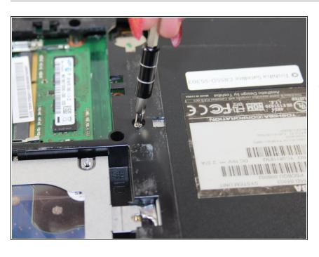
Locate the screw to the right of the RAM inside the panel. This screw is 6mm long (5mm head); remove it with a small Phillips head screwdriver.
