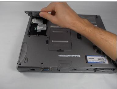
Unscrew the one Phillips #0 screw at the bottom of the panel and remove the panel.
