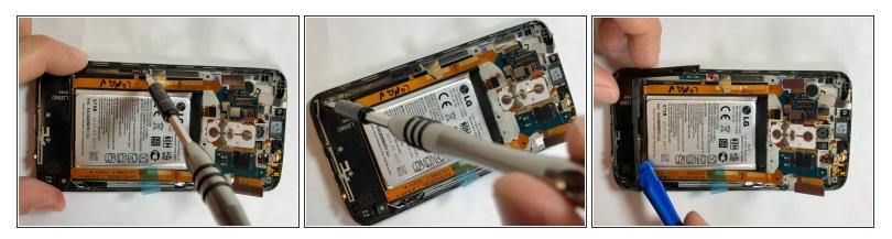
• The bottom inside panel should pry back easily after you take out the screws. Again, if the panel does not pull off easily, you may have missed a screw.
