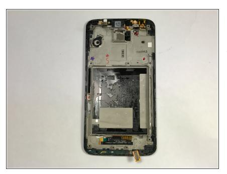
Once all components have been removed the display assembly with be the only part left, the final step is to replace this part.
