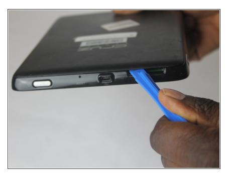
Insert the plastic opening tool in the SD port. The edge point should be pointed towards the rear panel.
