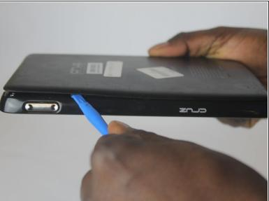
Move the small tool opener around the rear panel to free the 12 edges.
