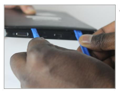
Insert a small opening tool between the rear panel and the tablet.
