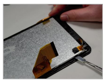
• With the motherboard and battery detached, use the Metal Spudger tool to gently remove the display from the front panel.
