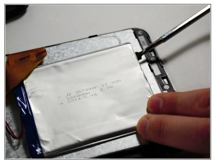
• Follow the guide to remove the battery from the back of the display.
