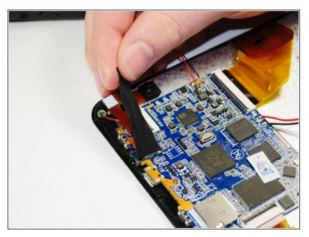
Remove black electrical tape to release the sensor and ribbon wires connecting the camera to the motherboard.
