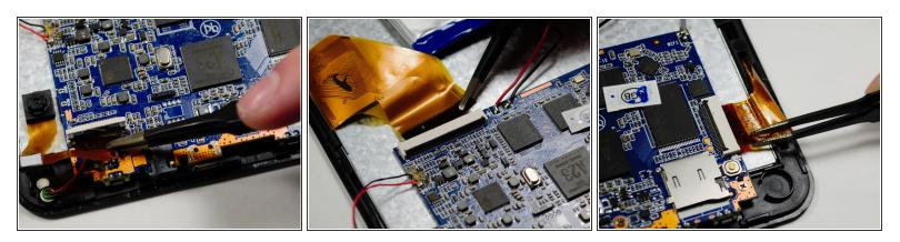
• Using a pair of the Precision Tweezers, remove the ribbon wire from the clip.
