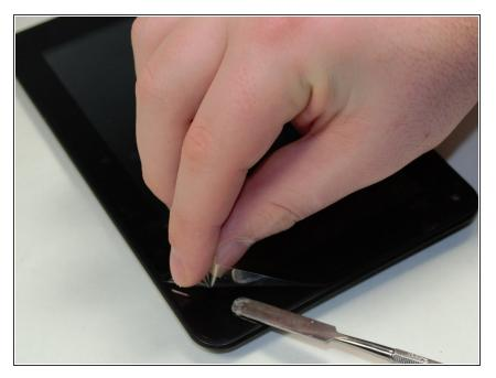
Use the Metal Spudger tool and your fingers to peel off any existing screen protector.
