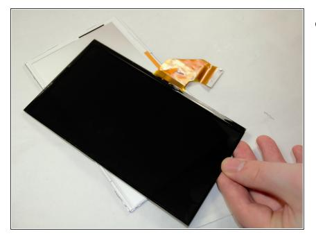
Remove the display from the plastic casing. The screen is now ready for replacement.
