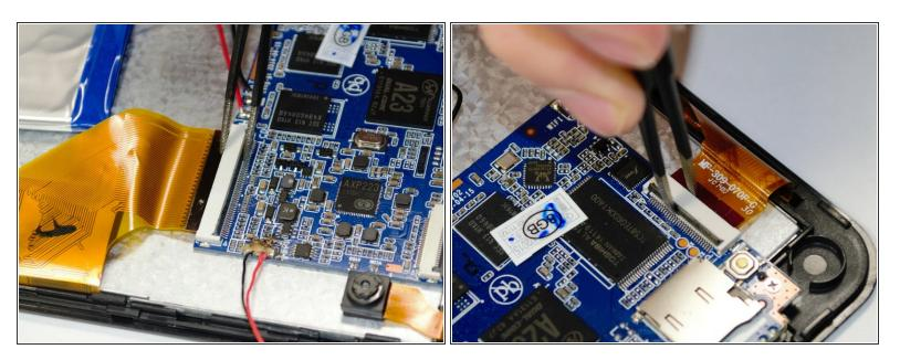
• Use a pair of Precision Tweezers to squeeze the clip of the ribbon wire to release it.
