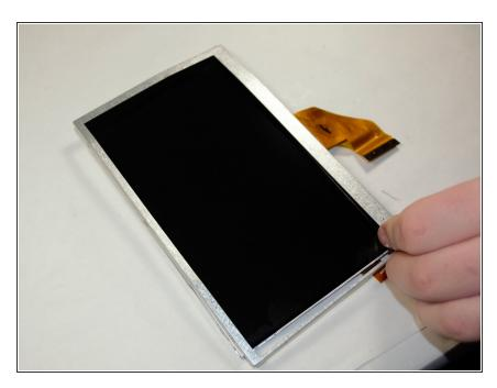
• Remove the LCD 5-Point Touch Screen from the display case.
