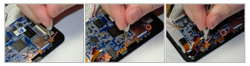
Use the #000 Phillips screw driver to remove all three 2.2mm screws attached to the mother board.
