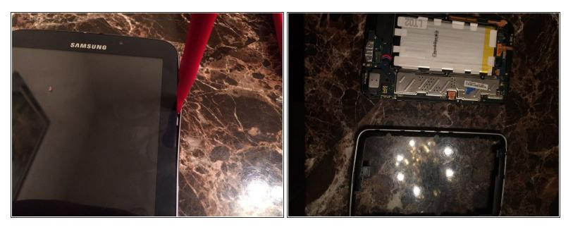
• turn it around then insert the mini pry bar between the screen and the silver border and slide the pry bar around all sides until the silver lining is poping off the screen
