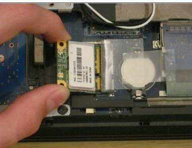
Just like RAM, hold the WLAN card by the edges and pull it out at an angle.
