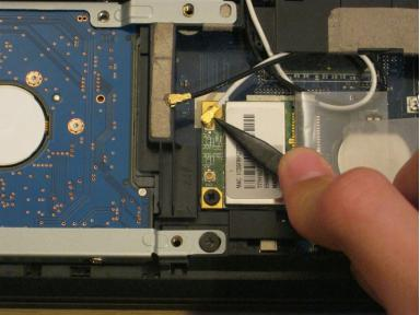
Use the pointy end of a spudger to remove the antenna connectors from the WLAN card.
