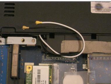
(i) You may find it useful to pull the antenna cables out from under the plastic retaining clip so you can move them out of the way while you work.
