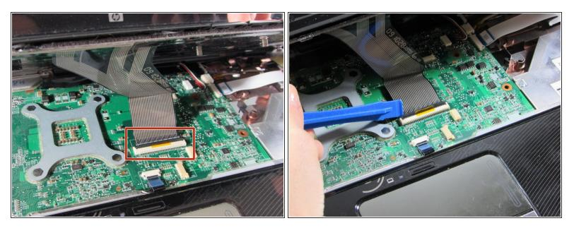
Use plastic spudger to flip up the black strip on the ZIF connector that connects the ribbon cable to the motherboard.
