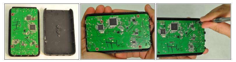
• Remove the four screws that hold the motherboard in place.
