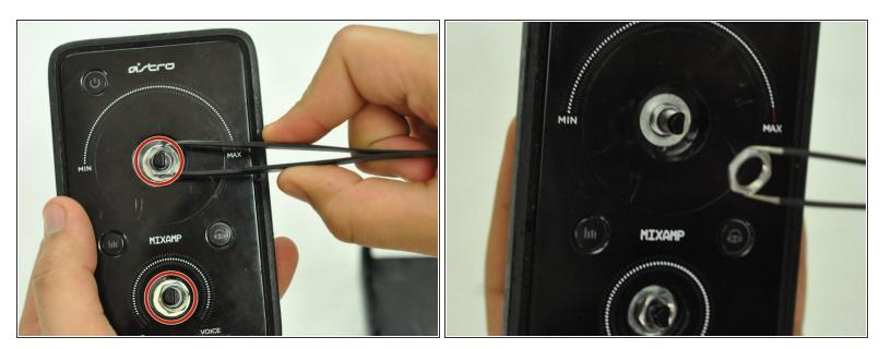
• Using tweezers, remove the spacer nuts and washers from each dial post.
