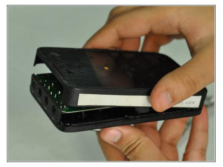
• Gently lift the rear casing from the device.
