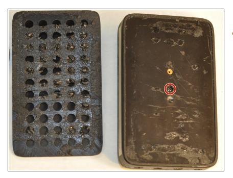
• Use a screwdriver to remove the screw from the rear casing.
