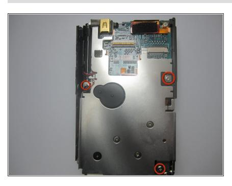
Remove the three 3.4 mm screws from the back side of the camera.
