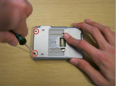
Remove the two Phillips #00 screws on the back of the device.
