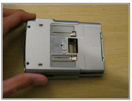
Using a spudger, gently separate the back casing from the rest of the device.
