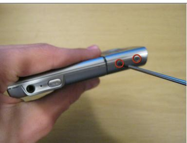
Remove the two Phillips #00 screws on either side of the device, on the sliding panel.
