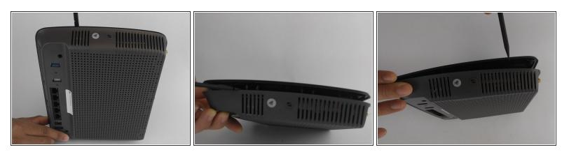
Depress the 12 clips along the edge into the router. Use the nylon spudger as using a metal object could cause damage.
