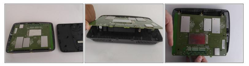
• Lift the board and pull down, away from the antennas.
