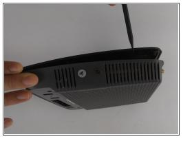
Depress the 12 clips along the edge into the router. Use the nylon spudger as using a metal object could cause damage.
