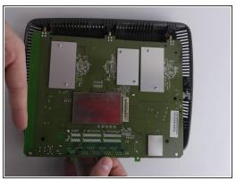
Lift the board and pull down, away from the antennas.
