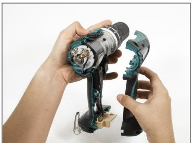
• Apply slight pressure to the sides of the outer casing and pull away from the drill.
