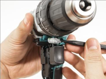
Use the pointed end of a plastic spudger to push the LED out of the drill.
