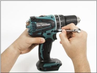
• Unscrew the nine 18 mm screws from the outer casing using a Phillips PH2 screwdriver.
