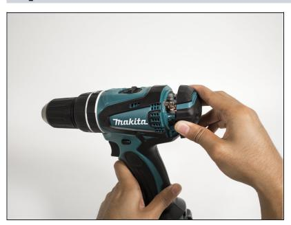
Apply slight pressure to the sides of the backplate and pull away from the drill.
