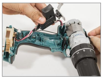
• Pull the black trigger assembly away from the drill.
