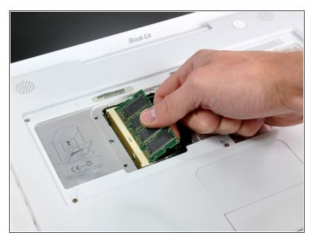
Pull the chip directly out from its socket.
