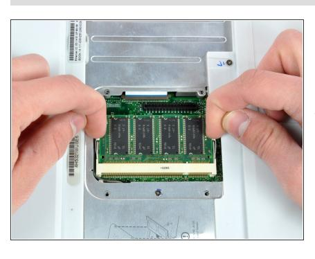
Release the tabs on each side of the RAM chip at the same time. These tabs lock the chip in place and
