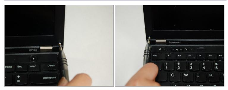
• Remove the screws (0.4, 0.5 cm) from the bottom corners of the bezel using a Phillips #0 screwdriver.
