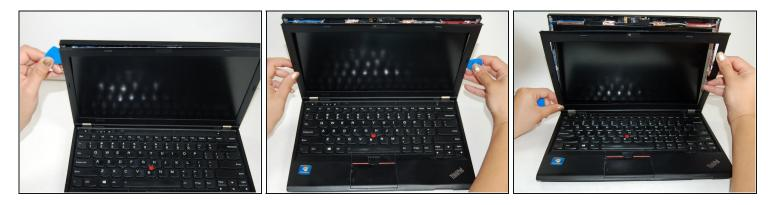
• Carefully remove the plastic bezel cover using an iFixit opening pick.
