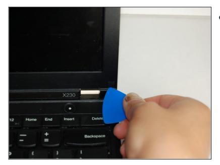
• Remove the plastic screw covers with an iFixit opening pick.
