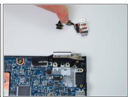
• Carefully slide bundle cable connector out from its connector on the motherboard.
