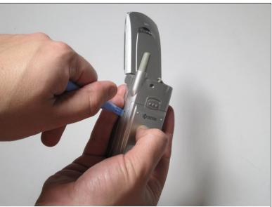
Wedge the opening device into the side crease of the phone.
