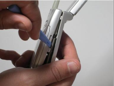
Slide the opening device downward to dis-join the rear casing from the front casing. Continue around all edges.
