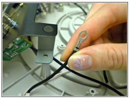
Remove the screw that connects the black wire of the tone arm to the base of the audio jack housing.
