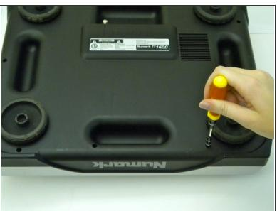
Flip over the turntable and remove the 9 screws on the outer edges.
