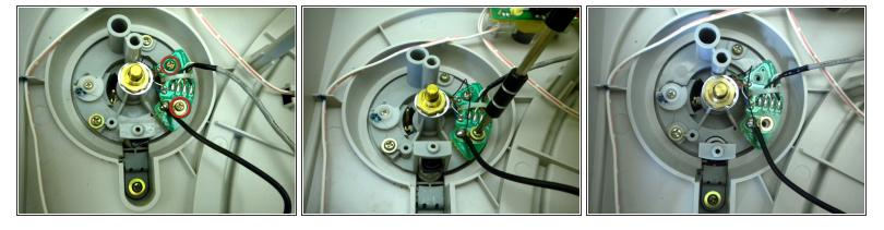
Remove the two screws connecting the circuit board to the tone arm.
