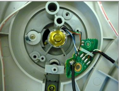
Remove the two remaining screws connecting the tone arm to the device.
