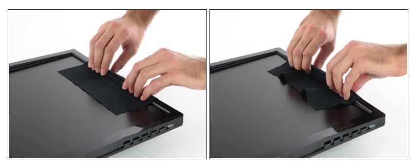
• Grip the center of the final side and lift the bezel away from the rear case.
