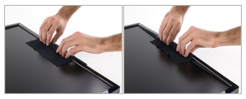
• Move around to the other long side and lift up on the center of the bezel.
