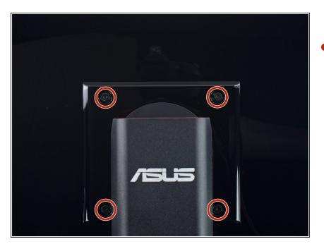
Remove the four 13.4 mm Philips #1 screws securing the monitor stand.
