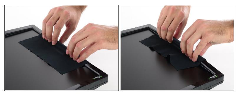
• Repeat the procedure around the display, lifting up the center of the next side.
