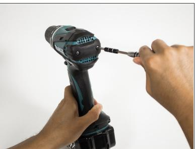
Unscrew two 18mm screws from the back panel with the Phillips PH2 screwdriver.
