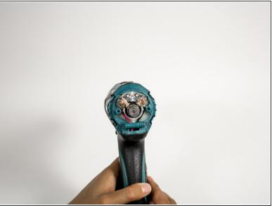
Apply slight pressure to the sides of the backplate and pull away from the drill.
