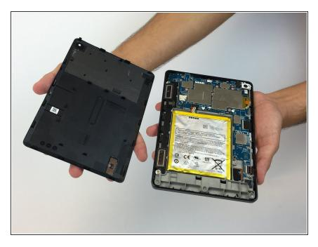
Once all clips have been released, remove the back case to reveal the inside of the device.
