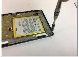
Following the bottom edge of the device, remove the (3) T5 hex silver screws with the T5 torx screwdriver.
