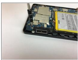
Remove the nine silver screws located around the motherboard with the T5 Torx screwdriver.
