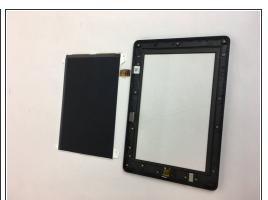
• The LCD display screen may now be removed and replaced.
