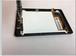
Remove the (4) T5 hex silver screws in the corners of the display screen using the T5 torx screwdriver.
