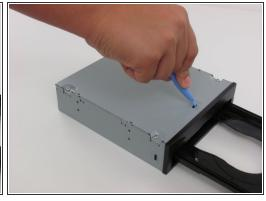
Use an opening device to push in the black tabs on the left, right and bottom of the outer chassis to unhook the faceplate.
