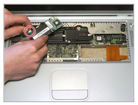
• Disconnect the connector cable from the modem.
