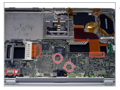
Disconnect the four indicated connectors from the logic board, removing tape as necessary.
