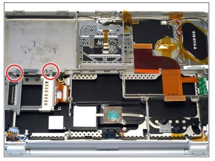
• Remove the two T8 Torx screws that secure the PC Card cage.
