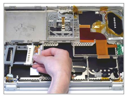
Remove the PC Card cage by pulling it to the right and twisting slightly toward you.
