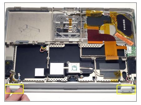
Close the display and pull off both clutch covers. You can use a nonmetal flathead screwdriver if the clutch covers do not come off easily.
