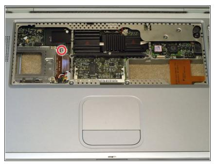
• Remove the single T8 Torx screw located next to the PC Card cage.
