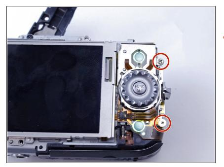
Remove two 3.2mm PH000 screws on the side of the camera, to the right of the button that reads "Func. Set."
