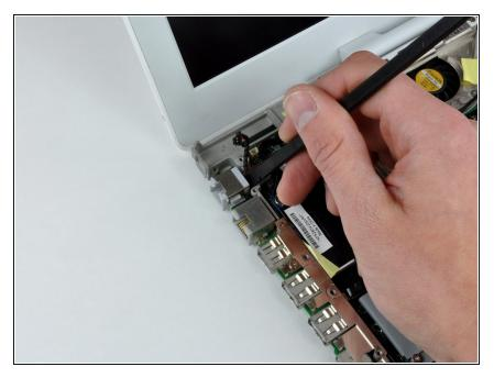
• Wedge a spudger between the RJ-11 board and the metal framework and slide the board off of the logic board.
