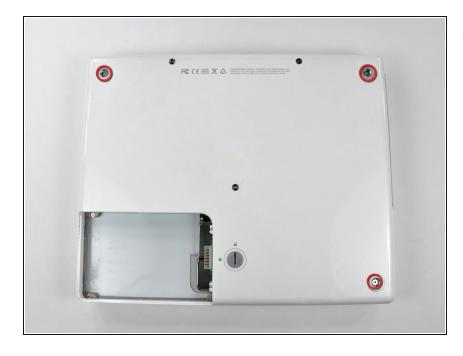
• Remove the three newly-revealed Phillips screws.
