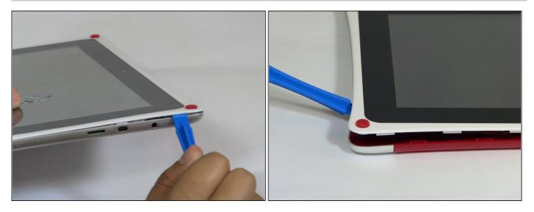
• Use the plastic opening tool at the top left corner seam, then pry the corner apart.
