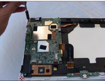
• Remove the four 4mm Phillips screws with the PH#0 screwdriver.
