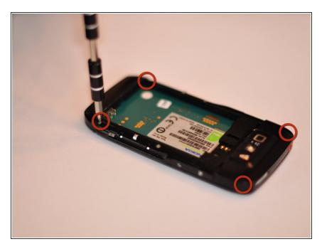
Using Torx number 4 unscrew the four 0.5mm screws.
