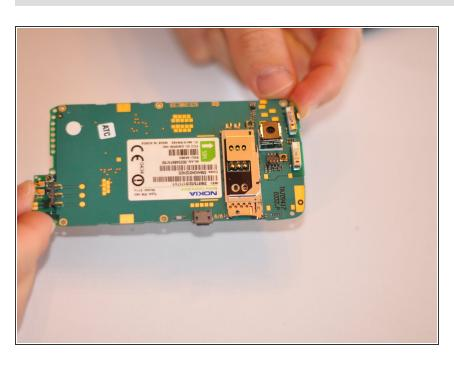
Replace motherboard, ensure that replacement has the same serial number.
