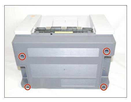
Using a Phillips #2 screwdriver, remove the four screws on the back of the printer.
