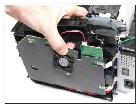
Poke out the side fan from the inside of the printer.
