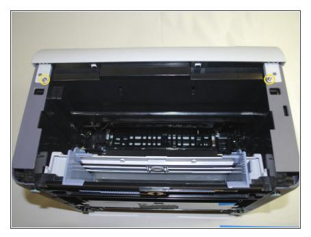
Using a Phillips #2 screwdriver, remove the two 1" screws on the front face of the printer.
