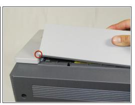
Remove the top hinged panel by taking out the pins at the bottom of this panel.
