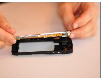
Once screws are removed detach back of phone from the motherboard.
