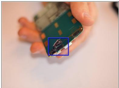
Carefully un-clip camera ribbon. Install new camera.
