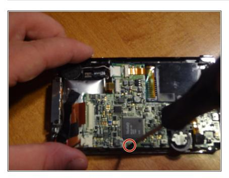
Remove one screw located on the board below the battery.
