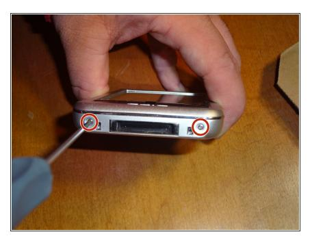
Remove two screws from the bottom of the device.
