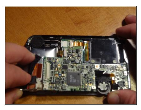
Unplug the male battery plug on the battery wire from the female battery plug on the board.
