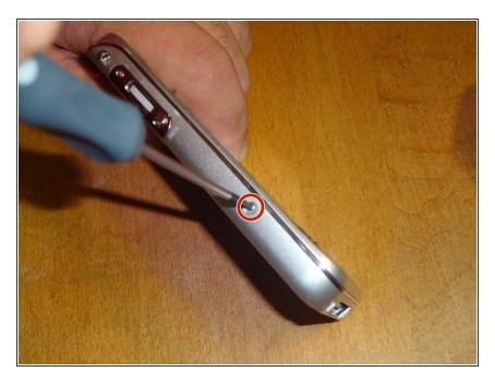
Remove one screw from lower right side of the device.
