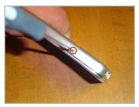
Remove one screw from the lower left side of the device.
