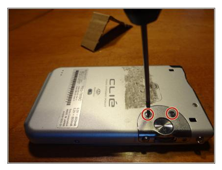
Remove two screws from the thumb dial panel on the back of the device.
