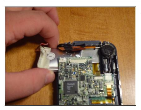
Remove the battery by sliding it out of the side of the device.
