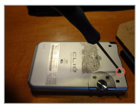
Remove one screw from the upper right corner on the back of the device.
