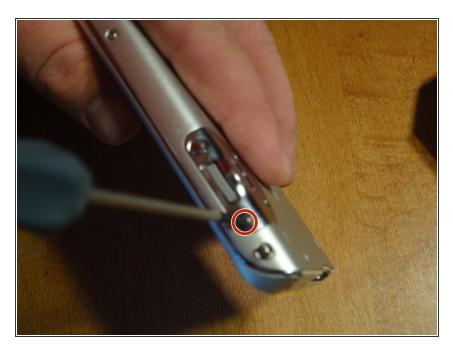
Remove one screw from the thumb dial panel on the right side of the device.
