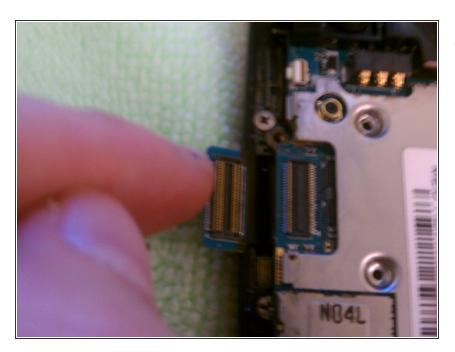
Use the ipod opening tool to disconnect the Connector
