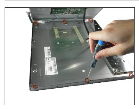
Remove the three 5.44 mm Phillips #00 screws on each side of the front of the metal casing.
