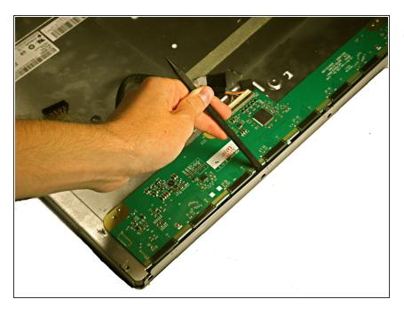
Use a spudger to pry the screen casing away from the metal casing.
