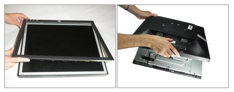
• When finished prying, the plastic will partially fall away from the rest of the monitor.
