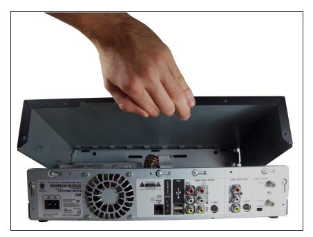
• Lift the cover up and off the device.
