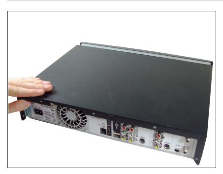
• Slide the cover towards the back until it is no longer under the front cover.
