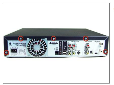
Unscrew the five 0.31 inch T-9 screws on the back cover.
