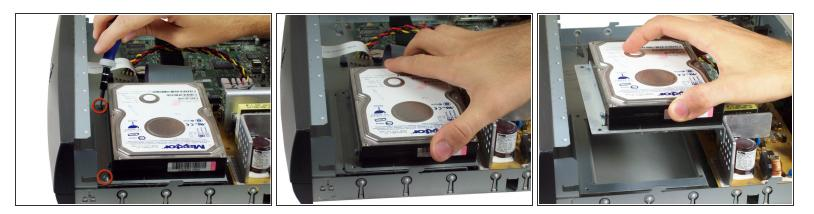
• Unscrew the 0.31 inch T-9 screws from the hard drive and pull outwards to remove.
