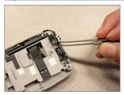
• Use the <u>tweezers</u> to remove the vibrator module.
