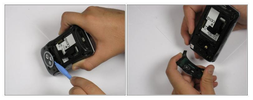
• Use a plastic opening tool to remove the camera cover.
