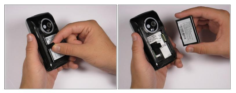
• Pull on the plastic tab to release the battery.
