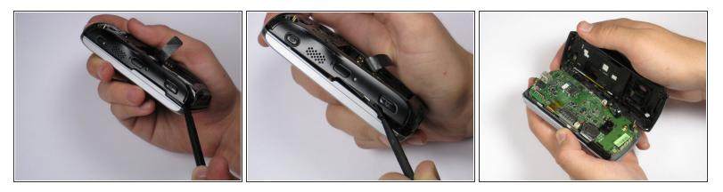
Be Careful! Do not insert the spudger in between the keyboard and screen. This could break the keyboard off the phone.
