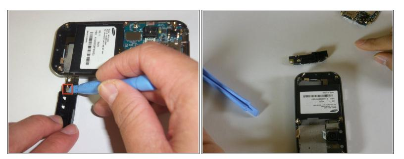
• Using a plastic opening tool, disconnect the connector leading from the antenna to the phone.
