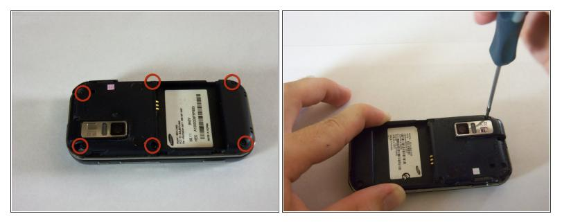
• Using a Phillips #00 screwdriver, remove the six 4mm screws holding the back case together.
